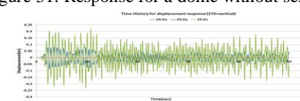
Figure 32: Response for a dome without seismic isolation system (270+vertical, t=10.77)
