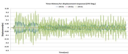
Figure 28: Response for a dome without seismic isolation system (270 Deg., t=10.77)
